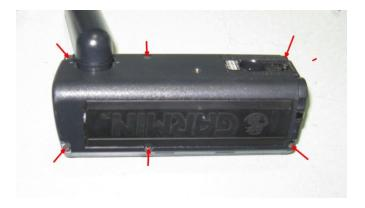
b. Carefully open the case. There is a connector cable that you can damage if it suddenly pops open.
