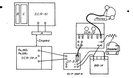
Fig. 63.—Cording diagram of connections when operating the SCR-54-A, the DT-3-A, and the SCR-72 sets together.
