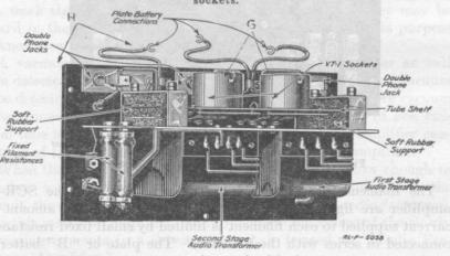
Fig. 61.-Panel of set box BC-17 removed to show interior parts.
