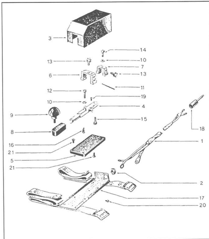
Fig. 4. Key and Plug Assemblies, CDN, No. 9. Type 1 (ZA/CAN 1643),
