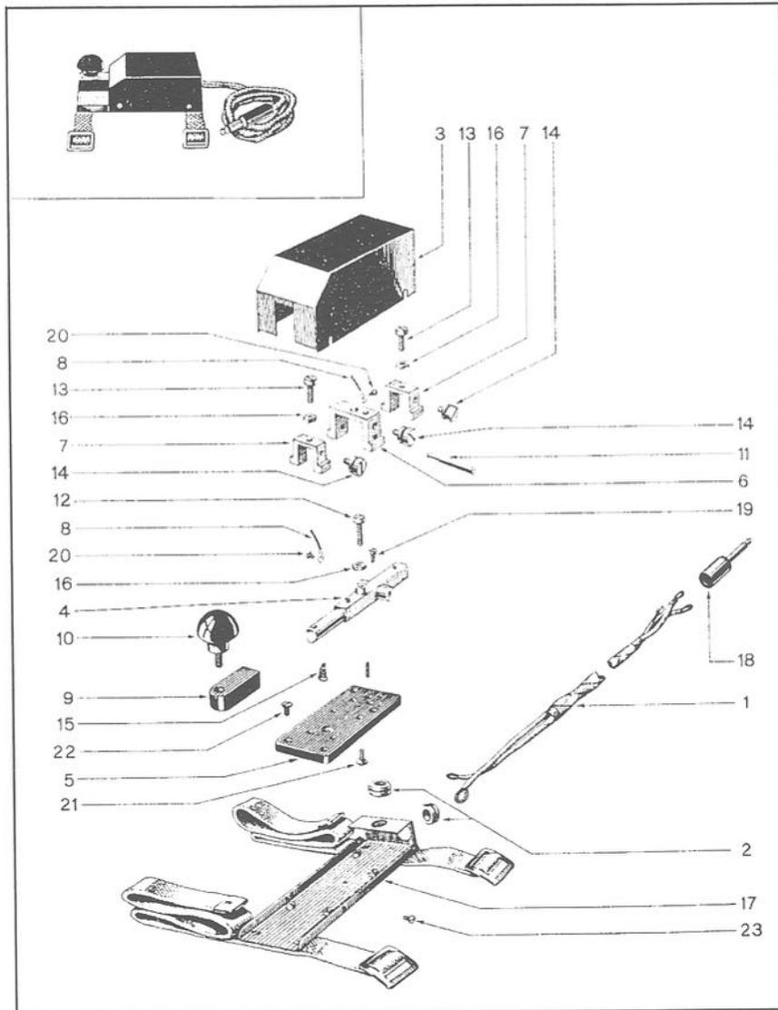
Fig. 1. Key and Plug Assemblies No. 9 (ZA/CAN/BR 0937),
