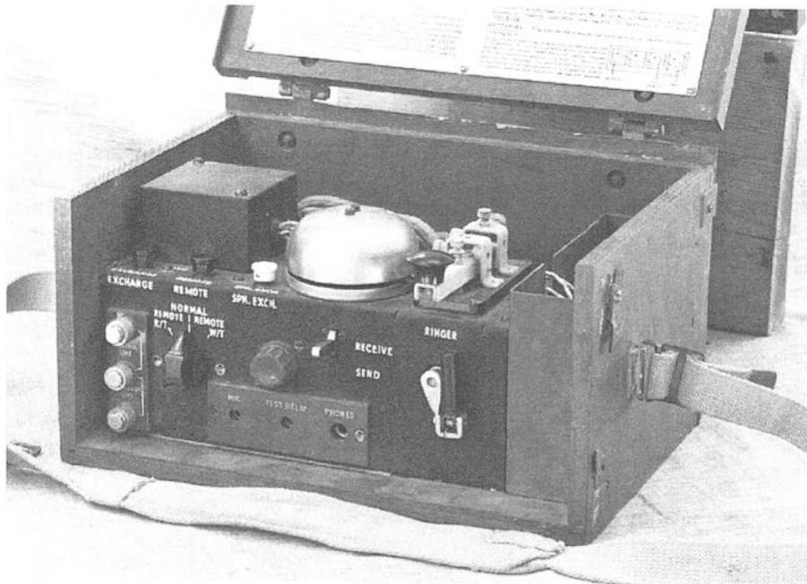
Fig. 8. Keys, W.T. 8 Amp, No. C1 (ZA/CAN 0977) as used in Wireless Remote Control Units, CDN, No. 1 (ZA/CAN 1332), also shown below in close-up
