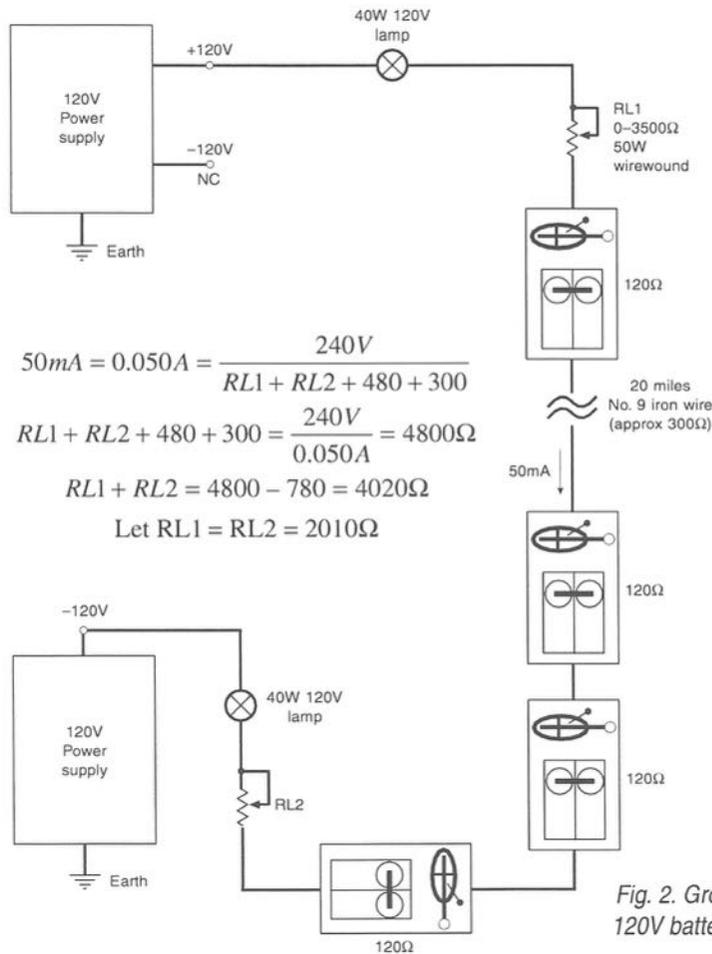
Fig. 2. Ground return circuit – 120V battery feed at each end
