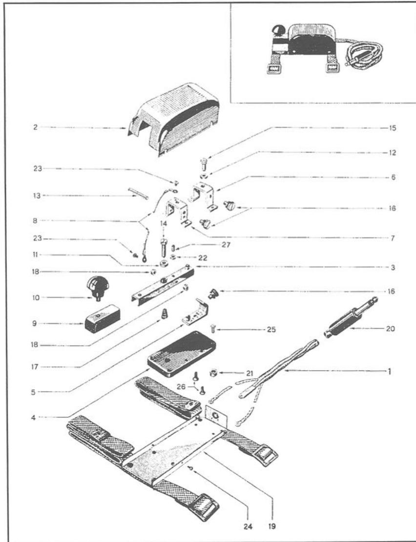
Fig. 5. Key and Plug Assemblies, CDN, No. 9 Type 2 (ZA/CAN 0715),
