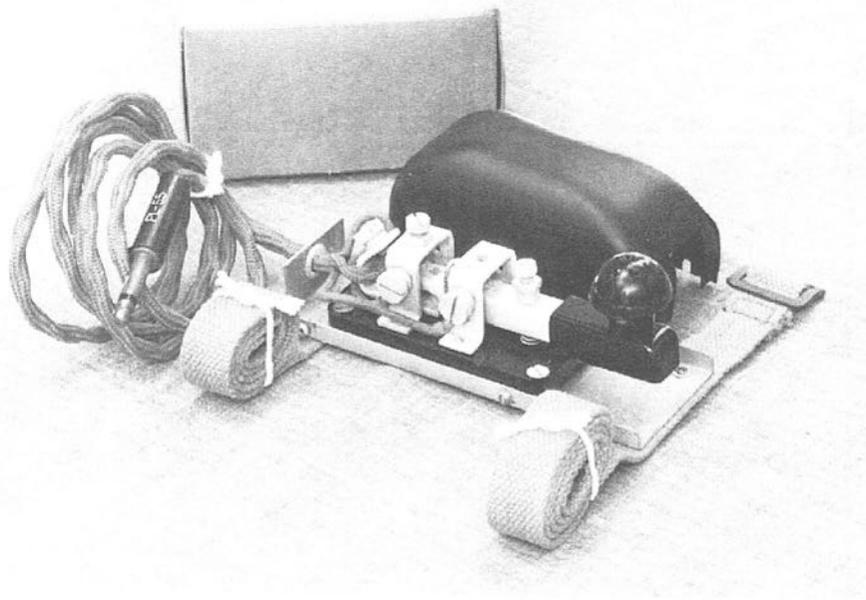
Fig. 6. Key and Plug Assemblies, CDN, No. 9 Type 2 (ZA/CAN 0715)
