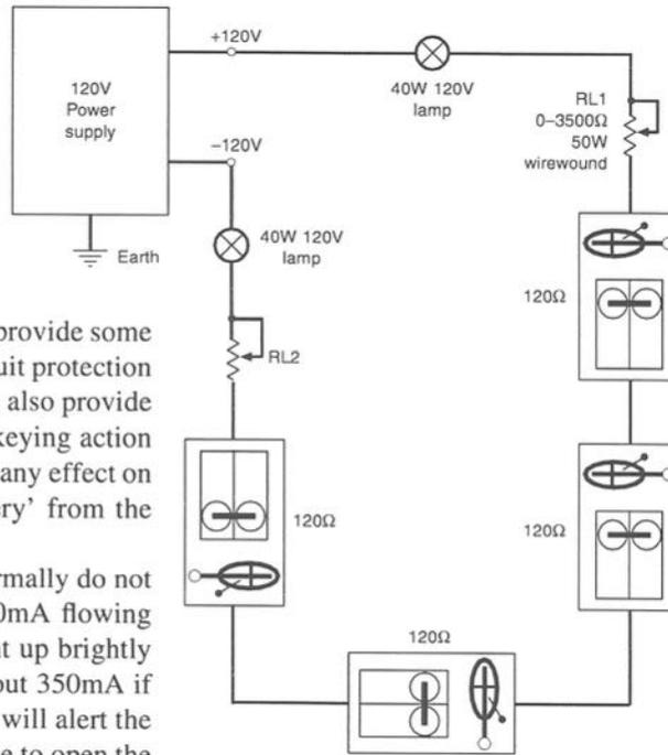
mon light bulb) in order to provide some over-current and short-circuit protection for the circuit. These lamps also provide some isolation so that the keying action of one circuit will not have any effect on other circuits 'taking battery' from the same voltage supply.
