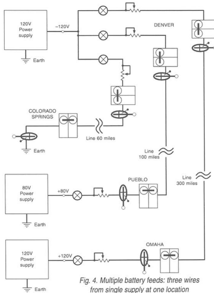
Fig. 4. Multiple battery feeds: three wires from single supply at one location
