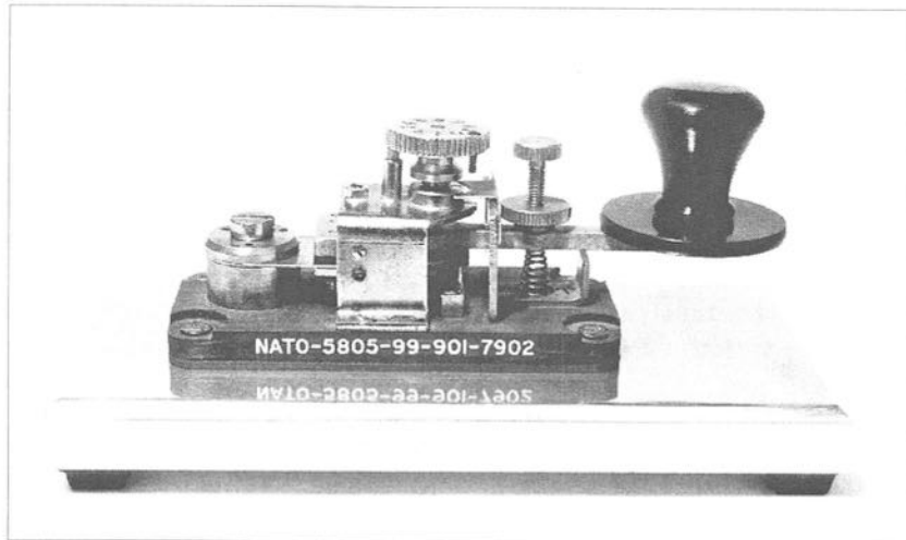
NATO-5805-99-901-7902 key with cover removed to show detailed construction
