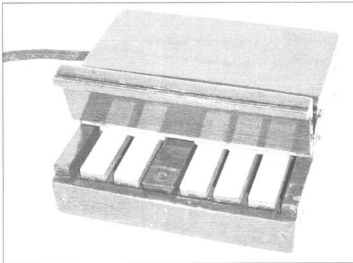
Keyboard for Baudot telegraph (1870's). The Frenchman Emile Baudot devised his telegraph so that he could apply a mechanical time division multiplier allowing to concentrate up to 6 stations on 1 line. This was possible by using a 5 element /character code (forerunner of the teleprinter code !), therefore the 5 keys on his transmitter.
