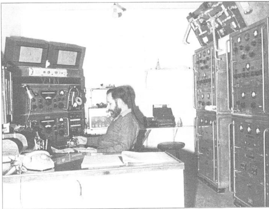
Macquarie Island 1969. Ray Langtip sending Morse traffic seated in front of Collins receivers. Behind are two AT20 transmitters.
