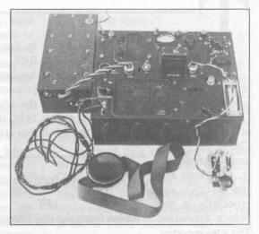
SOE's compact A Mk III transmitter-receiver built by the Marconi Company. Sometimes known as the B-2 Minor, it fitted in a case measuring 13 by 9 by 4in. about the same size as the Special Communications Mk VII/B ('Paraset')
