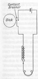
Fig. 4. Omnigraph circuit with buzzer From Harmsworth's Wireless Encyclopaedia
