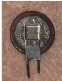
1. Replacing the battery. If you do not have the equipment and ability to do fine soldering do not attempt this project. Please note that removing the backup battery will delete all waypoints and other stored information.
