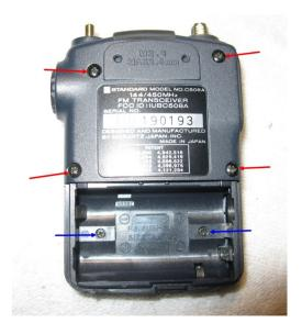
5. Gently pull the two case halves apart, starting from the bottom end. Locate the ribbon cable inside the case. It can tear, so be very careful with it.
