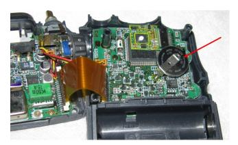
7. Using a fine soldering tip, touch it to each battery solder pad while lifting the contacts gently with a pair of tweezers. Do this as quickly as possible. The battery is sitting on a foam pad that will melt if you are not careful. The pad is stuck to the battery with adhesive, so you will have to pull it off.
