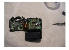
6. Lay the halves next to each other on a soft surface. Locate the battery.
