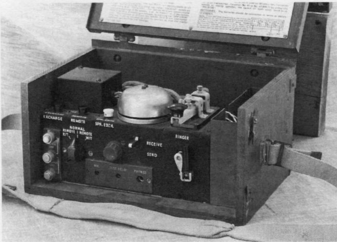
Fig. 8. Keys, W.T. 8 Amp, No. C1 (ZA/CAN 0977) as used in Wireless Remote Control Units, CDN, No. 1 (ZA/CAN 1332), also shown below in close-up
