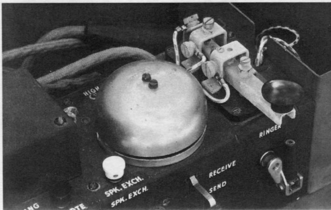
Fig. 8. Keys, W.T. 8 Amp, No. C1 (ZA/CAN 0977) as used in Wireless Remote Control Units, CDN, No. 1 (ZA/CAN 1332), also shown below in close-up
