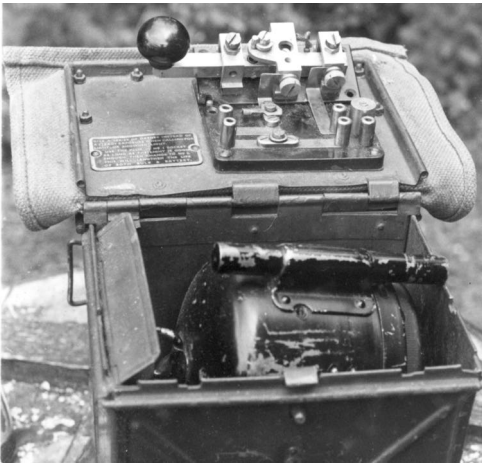
Key WT 8 Amp No2, LMK 1939, fitted on Lamp Signalling Daylight Short Range Projector MKII. Photo: Malcolm Henchley G0CHZ.
