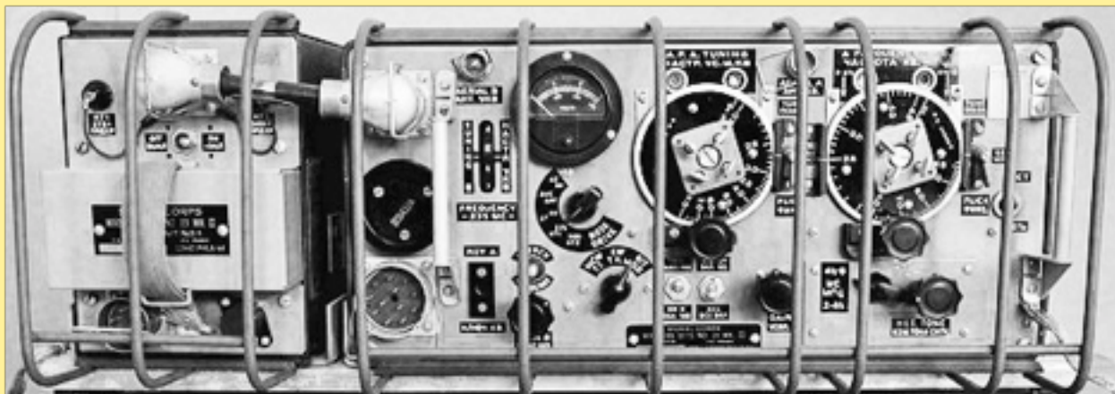
Wireless Set No.19. Workhorse of the Allied Forces in WW2 and later. The natural partner of the Key WT 8 Amp.
