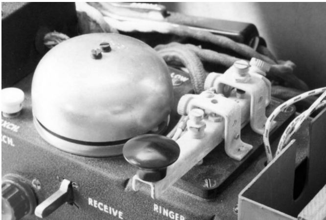
Key WT 8 Amp No C1 (ZA/CAN 0977) used in Wireless Remote Control Unit CDN, No.1. Note knob, specific to this version. Photo: Chris Bisailion VE3CBK.
