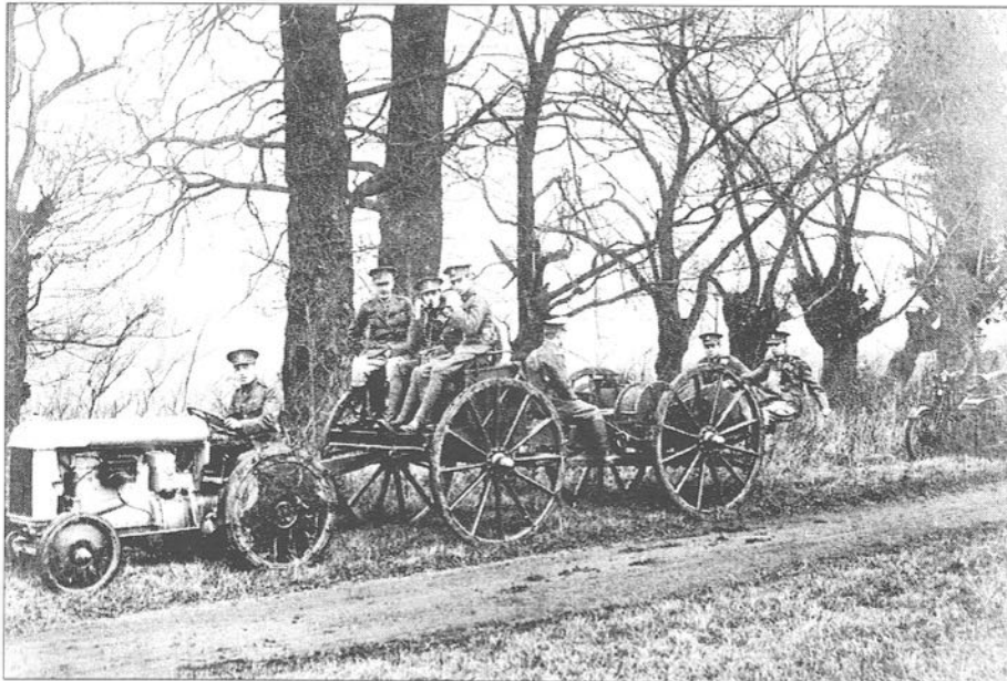
Figure 6. Cable wagon drawn by a tractor. Museum of the Royal Corps of Signals
