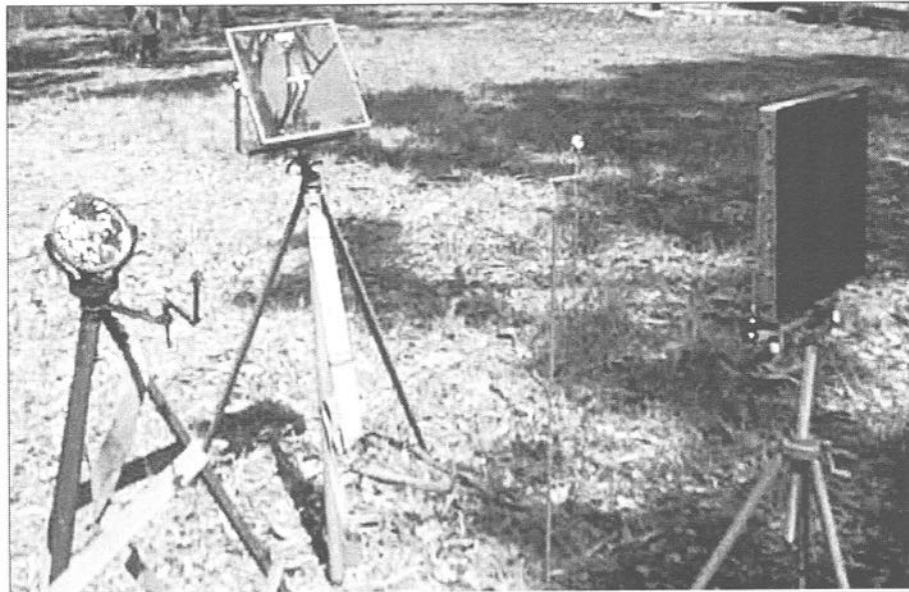
Figure 1. Left: British army pattern Mk V heliograph with tilting mirror. Right: Home made heliograph constructed to the American pattern with louvered shutter.
