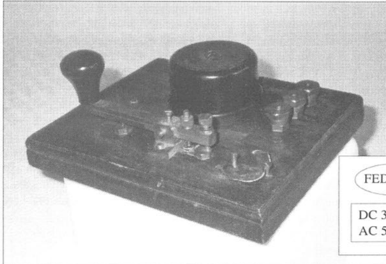
Small brass 'Gamage' type of key on a base with three unusual terminals and buzzer marked as shown in the inset.
