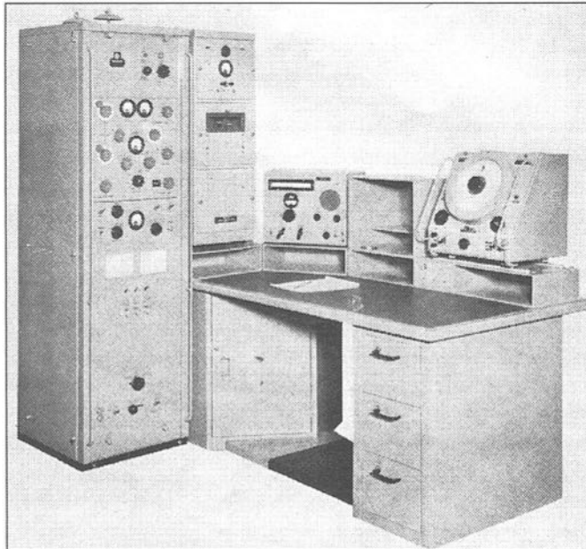
Marconi "Oceanspan" CW/ICW Transmitter (medium and short wave); "Yeoman" All Wave Receiver; "Vigilant" Auto Alarm and "Lodestone" Direction Finder as fitted at the School.
