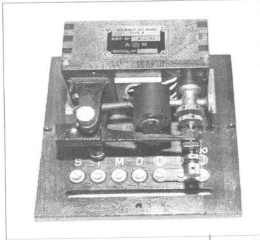
Photo/Collection: Stan Barr GØCLV Above - Sounder Relaying Type A, Ref: 10G/117. It comes with a glass topped case.
