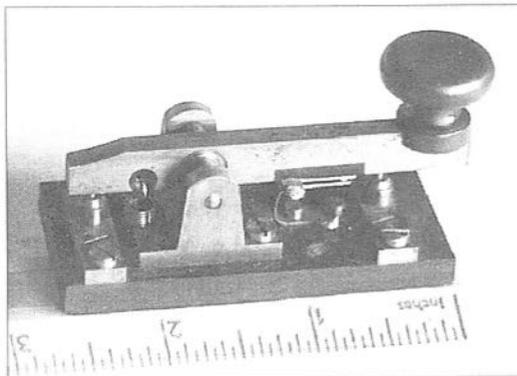
Small key, just over 2 1/2 inches long, bought in Prague recently. Has an additional contact under the lever (insulated from the rest of the key) which closes just before the front contact. Mike Kerr, ZL2BCW, says: 'The metal work is finely executed and the lacquered brass has that patina that is only acquired over a considerable period of time. The knob and base are ebonite or hard rubber perhaps. There are no markings of any kind'. Info requested
