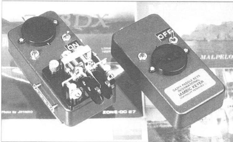
Use it as a Combo, or use the key on its own, or the Iambic keyer on its own. Incorporating the TiCK-2 keyer chip from Embedded Research, with paddle or push-button control of speed, message memory, paddle selection, iambic mode, etc.
