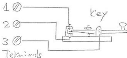
It was used on Japanese ships c.1929–1945. The terminals are numbered 1 to 3, connected as illustrated, and were used for break-in operation with MF and HF transmitters.
