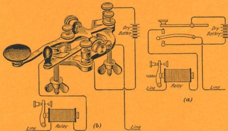
**Fry, Open-Circuit, Dry Battery, Telegraph Key**
