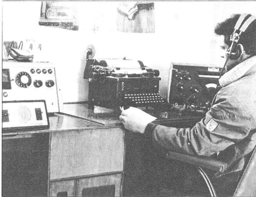
1965 – Allan Moore at Mawson's 2nd Morse position. Left is an auto-dial unit for the 5kW transmitter and selector switches for other remote transmitters. Centre is a single-case typewriter for copying CW. Right is a Collins 51J-4 receiver and old Vibroplex bug on the desk
