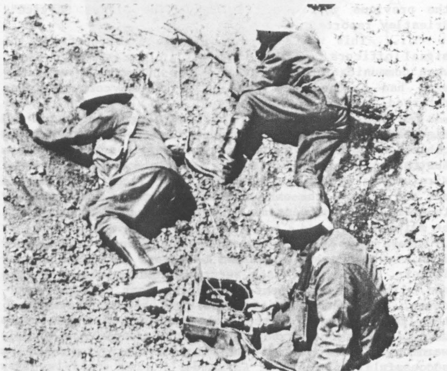
Fig. 2. The Power Buzzer used for one-way signalling from an advanced observation post back to H.Q.
