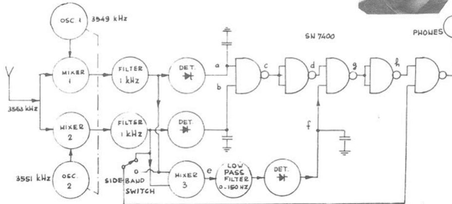
= Direct conversion reception without the disadvantage of hearing the signals both sides of the beat frequency =
